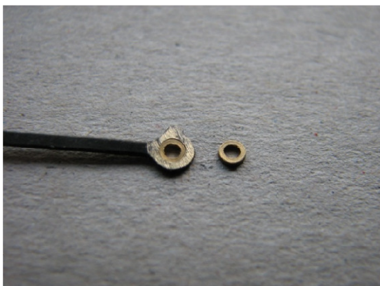
Bush in rod ready for soldering.
